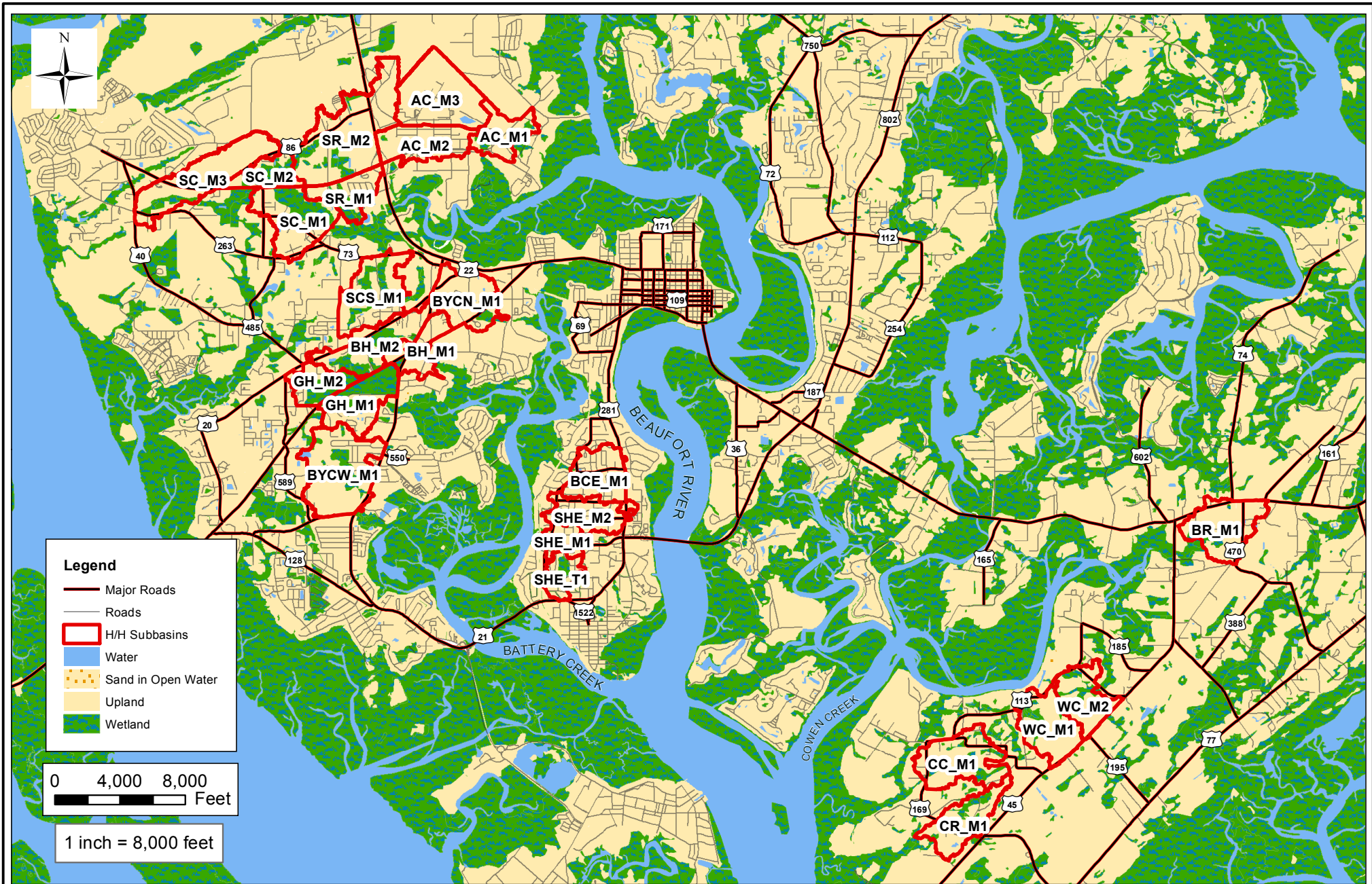
Figure 8-2. Hydrologic Model Subbasins Beaufort River Watershed
